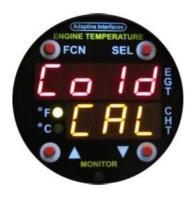
TO PERFORM THIS SETTING, BOTH THERMOCOUPLES NEED TO BE REMOVED FROM THE ENGINE AND PLACED IN AN ICE BATH AT 32° F.
