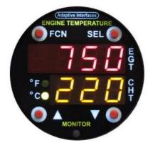
In this mode, Exhaust Gas Temperature and Cylinder Head Temperature are displayed in METRIC units. EGT and CHT are displayed in Degrees Celcius.
