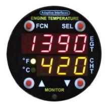
In this mode, Exhaust Gas Temperature and Cylinder Head Temperature are displayed in ENGLISH units. EGT and CHT are displayed in Degrees Fahrenheit.
