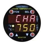
The CHT HIGH TEMPERATURE ALARM can be cycled OFF and from 500 °F to 900 °F in 10 °F steps.
