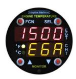
The EGT HIGH TEMPERATURE ALARM can be cycled OFF and from 800 °F to 1900 °F in 10 °F steps.
